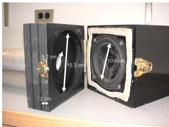
FIG. 5. (Color online) Close-up of the coupling of the speaker to the tube with relevant dimensions.
